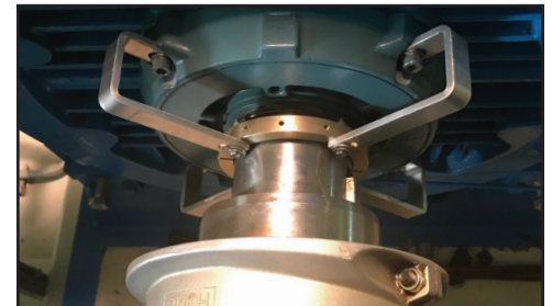
The Smart CDR can be installed with a variety of mounting configurations, including press-in, clip-on, epoxy, bolt-through, side-mount and flexbracket.
