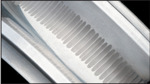
Stray shaft currents can cause fluting on the bearing race, resulting in premature bearing failure
