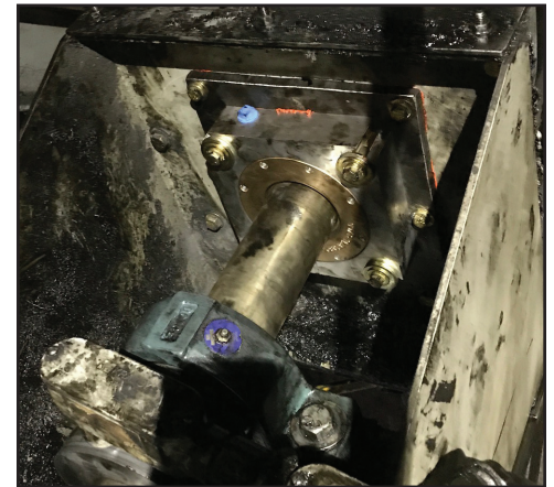
Air Mizer AM CEMA shaft seal installed on a CEMA Screw Conveyor.
