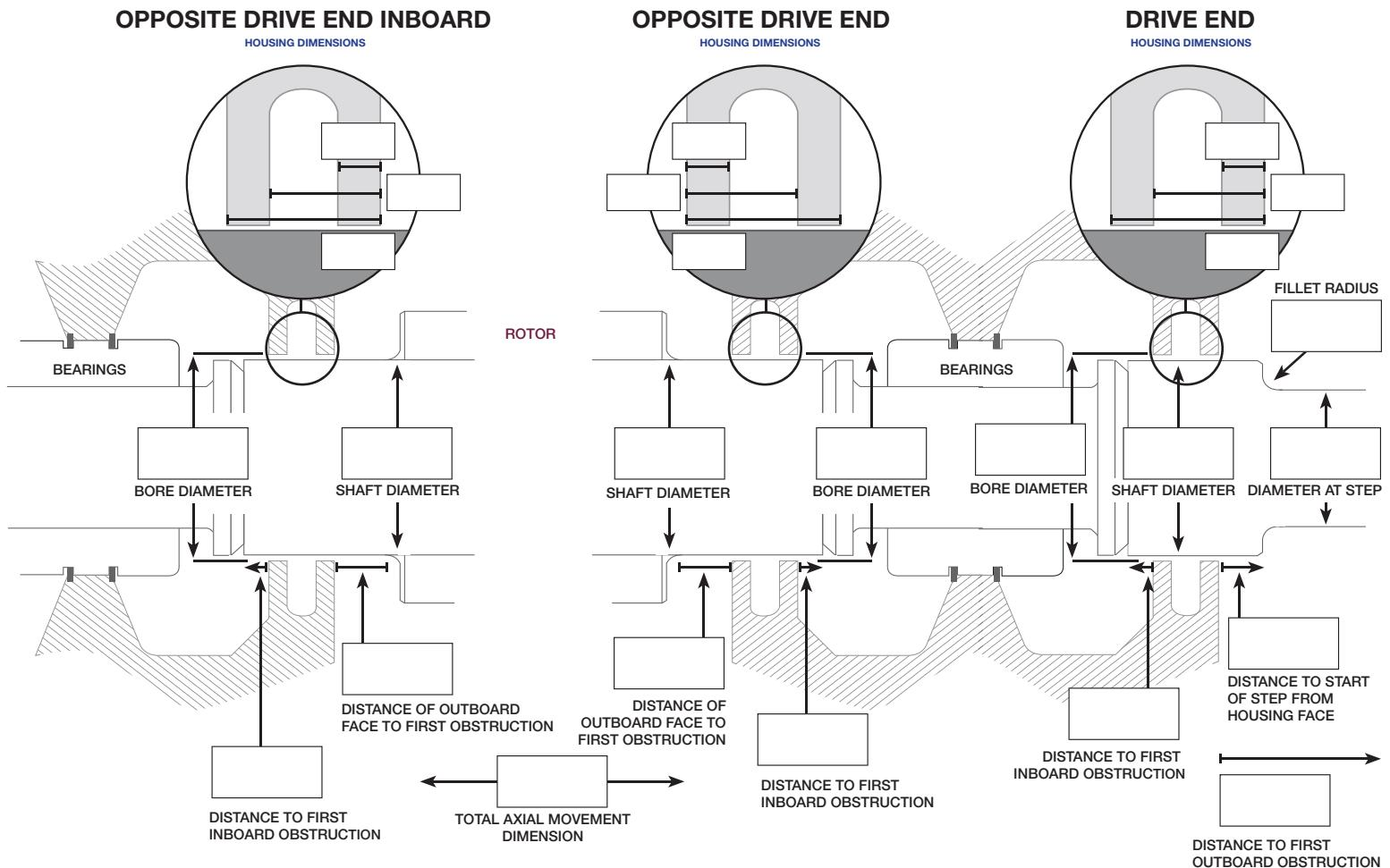
**AXIAL MOVEMENT DIMENSION WITH ROTOR THRUSTING TOWARD:** ODE DE
