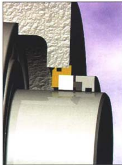
Fig. 4. Finite-life lip or face contact seals can be easily damaged during installation.
