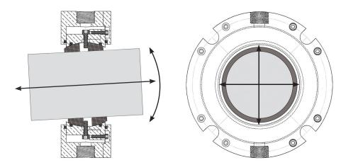
Inpro/Seal Air Mizer shaft seals are designed to handle extreme conditions including radial run-out, axial movement and angular misalignment simultaneously.
