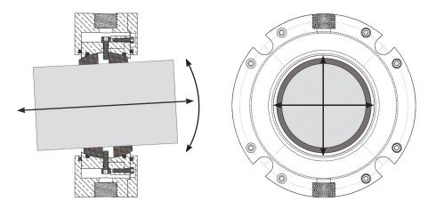
Inpro/Seal Air Mizer shaft seals are designed to handle extreme conditions including radial run-out, axial movement and angular misalignment simultaneously
