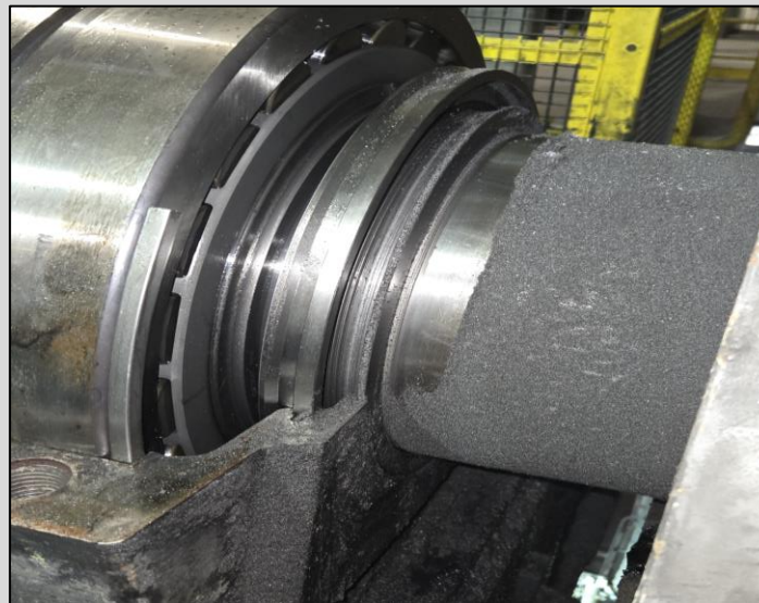
Before: Aluminum slag entering the pillow block bearing housing via a faulty taconite seal
