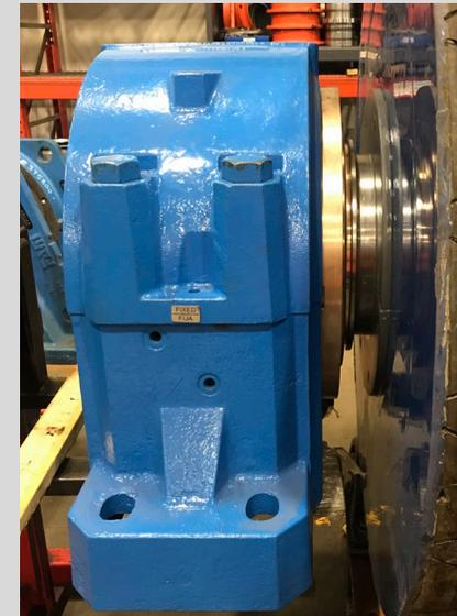
Inpro/Seal Bearing Isolator installed on SDCD 23176 Pillow Block
