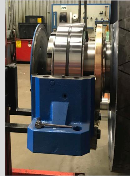
Inpro/Seal Pillow Block Bearing Isolator Installation
