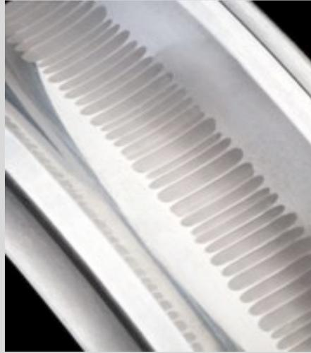
Electrical Discharge Machining (EDM) on the bearing race
