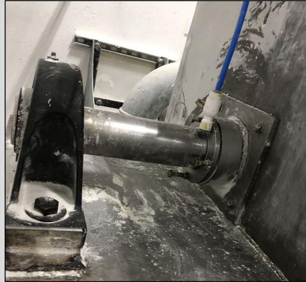
**Before:** Leaking ribbon blender showing air purged stuffing box.
