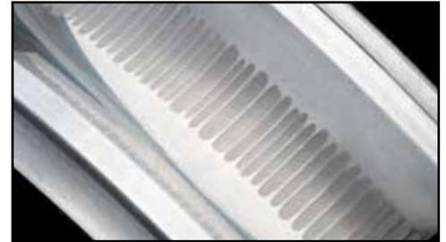
*Stray shaft currents cause fluting on the motor bearing race, resulting in premature bearing failure.*
