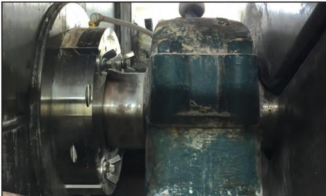
The Inpro/Seal AM Solutions shaft seal uses a positive purge of air along the shaft to permanently seal against product loss.
