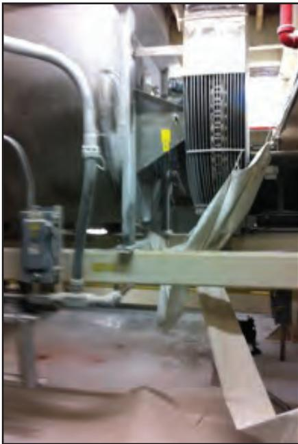
A bag catches pancake mix leaking from a mixer due to failed shaft seals, while additional leaking mix piles up on the ground.
