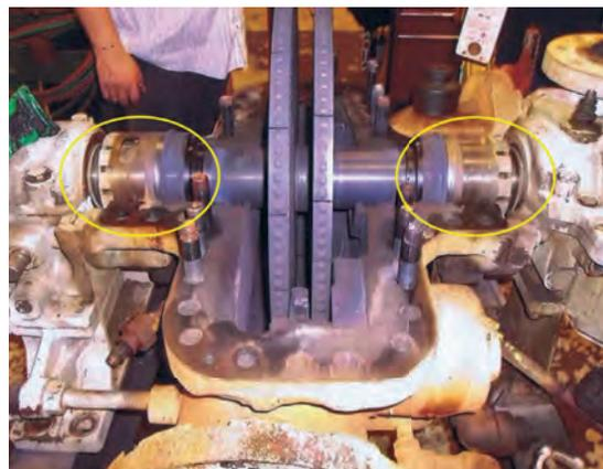
Machined gland boxes with a mechanical seal assembly
